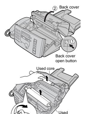
**3** Pull up the blue gear side and remove the used ink film. Remove the used core.
