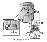
3 Insert the hooks on the wall mounting adaptor into holes (a) and (b) on the base unit.
