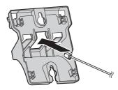
2 Tuck the telephone line cord inside the wall mounting adaptor (①). Connect the AC adaptor cord and telephone line cord (②).
