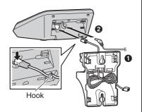
Insert the hooks on the wall mounting adaptor into the holes (A) and (B) on the base unit.
