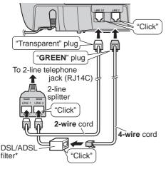
\*DSL/ADSL filter (not supplied) is required if you have DSL/ADSL service.
