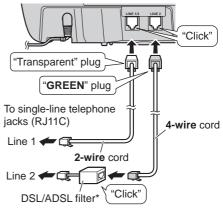
\*DSL/ADSL filter (not supplied) is required if you have DSL/ADSL service.
