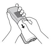
2 Insert the battery (●), and press it down until it snaps into position (②).
