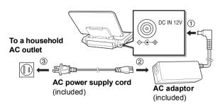
The unit is in the standby condition (the [ $\bigcirc$ ] indicator lights) when the AC power supply cord is connected. The primary circuit is always "live" as long as the AC adaptor is connected to an electrical outlet.
