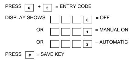
This code allows the system primary pump to be turned on, off, or put on automatic. The system primary pump circulates water from the boilers through the building. To use this code, enter 65, and then enter 0 or 1 to turn it off or on, respectively, which takes control of the pump away from the panel. Enter 2 to have the panel control the system pump. Please note that the pump must have an auto-reset feature to work with setting number 2.
