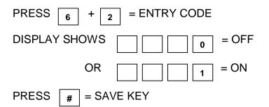
The system mode turns the boiler system off and on, and is commonly used to shut it down at the end of the heating season and turn it on again in the Fall. When turning the system on, the panel takes over control of the boilers, and in some cases the primary system pump. To use this code, enter 62, and the display will show either 0 or 1, for off or on, respectively. Enter your choice and press # to save.
