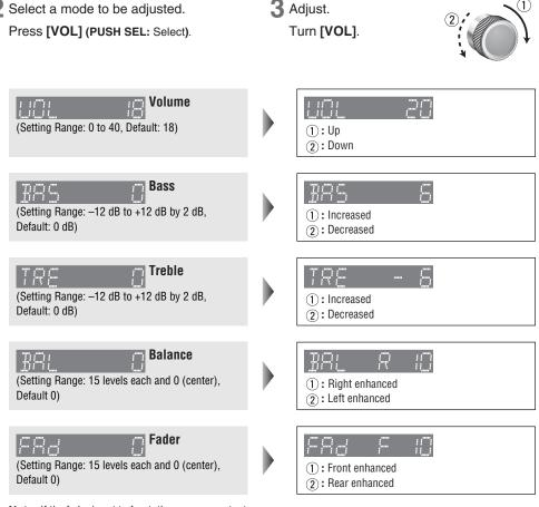
Note: If the fader is set to front, the pre-amp. output (rear) is decreased.
