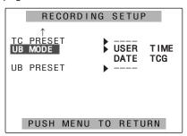
**3** Tilt the OPERATION lever in the ▼ direction and move to the **UB PRESET** item.
