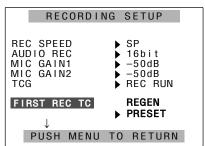
**3** Tilt the OPERATION lever in the ▼ direction and move to the **TC PRESET** item.
