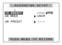
5 The screen shown below appears. Set the time code value using the OPERATION lever.
