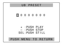
**6** Upon completion of the user's bit setting, press the MENU button. The screen shown below appears. Tilt the OPERATION lever in the ▼ direction, select YES, and press "I" of the OPERATION lever.
