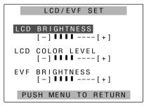
6 Select the LCD COLOR LEVEL item, and tilt the OPERATION lever in the ▲ or ▼ direction to adjust the screen's color level. (If the remote control unit is used, press the "►" button among the SET buttons.)
