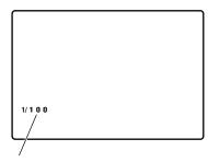
If a setting other than OFF has been selected for the OTHER DISPLAY item on the setting menu DISPLAY SETUP screen, the current shutter speed setting is displayed in the viewfinder and on the LCD monitor. However, it is not displayed if the standard (OFF) shutter speed has been set.
