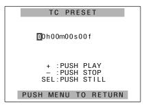
**6** Upon completion of the time code value setting, press the MENU button. The screen shown below appears. Tilt the OPERATION lever in the ▼ direction, select YES, and press "II" of the OPERATION lever.
