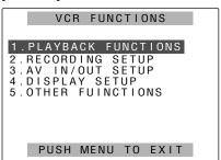
2 Tilt the OPERATION lever in the ▲ or ▼ direction, and move the highlighted part to the function which is to be set.
