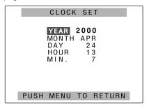
3 Tilt the OPERATION lever in the ▲ or ▼ direction and set YEAR to 2002. (If the remote control unit is used, press the "►" button among the SET buttons.)
