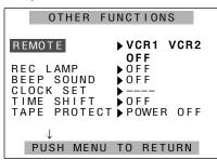
4 Tilt the OPERATION lever in the ▲ or ▼ direction, and move the highlighted part to the function which is to be set.
