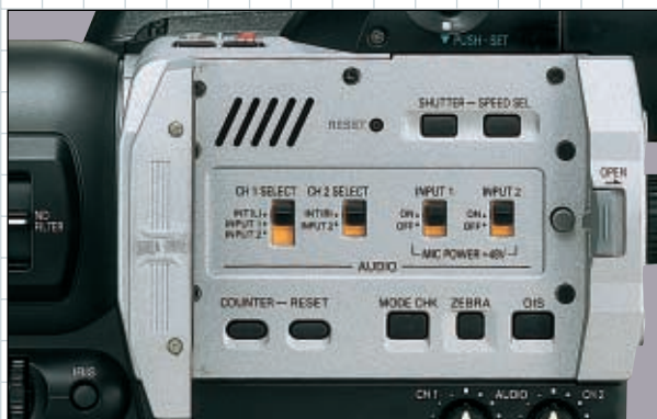
Sub-panel (with LCD monitor opened)
