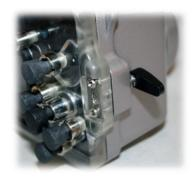
Pull out the lid by holding on the grip near the lock.
