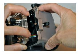
To close the housing, place the lid over the housing and align the key-hole and press down the lever.
