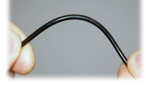
Once the O-ring has been inspected and verified fit for use, apply a small amount of silicone grease to the O-ring. The silicone grease must be evenly distributed round the O-ring. Install the O-ring into the groove; run a finger round the O-ring, to make sure it is snugly seated in the groove.
