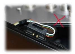
Replace the lid and make sure the lever is perpendicular to the side wall of the housing. Lock the lid by press down the lever and turn until the lever is parallel to the side wall of the housing.
