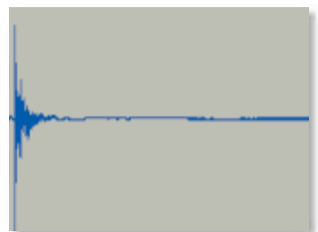
New Hybrid Aramid Speaker Cone (Resin/Long Fibers) Improved (higher) internal loss → Clarity of sound
