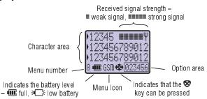
Following some operations the display will automatically clear after three seconds or after pressing any key except  $\infty$ .
