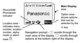
Following some operations the display will automatically clear after three seconds or after pressing any key.
