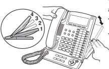
The tilt angle of the operation board can be adjusted to four steps-angles.
