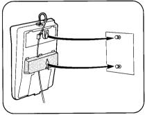
To temporarily place the handset down during a conversation, hook as shown.
