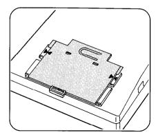
2 Push the two shaded portions slightly and insert the edges of the holder under the slide rails and then slide down toward arrow "A".
