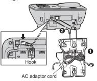
3 Insert the hooks on the wall mounting adaptor into holes (2) and (3) on the base unit.
