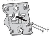
2 Tuck the telephone line cord inside the wall mounting adaptor (●). Connect the AC adaptor cord and telephone line cord (●).
