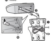
3 Insert the hooks on the wall mounting adaptor into holes **(a)** and **(b)** on the base unit.
