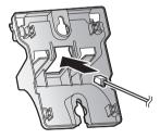
2 Tuck the telephone line cord inside the wall mounting adaptor (1). Connect the AC adaptor cord and telephone line cord (2).
