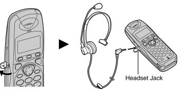
To adjust the headset receiver volume (HIGH, MEDIUM or LOW): While using the headset, press ♥ or ▲.
