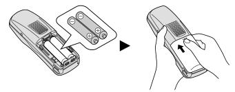
• If the rechargeable batteries are not inserted correctly, the handset will not work.
