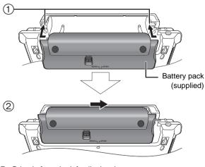
① Bring in from the left, aligning the grooves.
