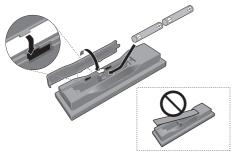
To close the rear lid, line up the catch with the groove and slide in the direction of the arrow  $(\Rightarrow)$ .
