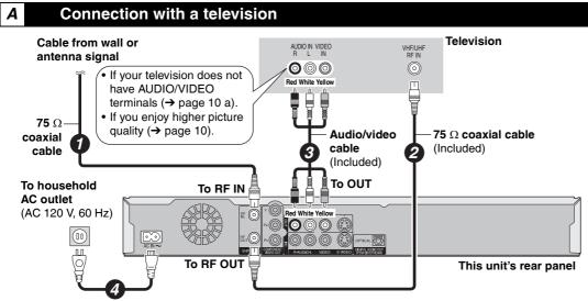
AC power supply cord (Included) Connect only after all other connections are complete.
