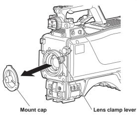
**2** Align the guide pin on the lens with the groove at the top center of the lens mount, and mount the lens.
