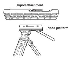
2 Mount the camera on the tripod attachment. Slide the camera toward the front along the groove until a click is heard.
