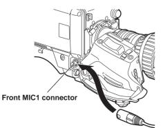
**4** If the audio channel whose signals are to be recorded so requires, set the MIC1 selector switch to FRONT MIC.
