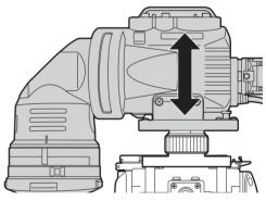
**3** Rotate the viewfinder forward/backward position fixing lever in the opposite direction until it locks.
