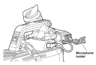
**2** Mount the microphone and tighten up the clamp screw.
