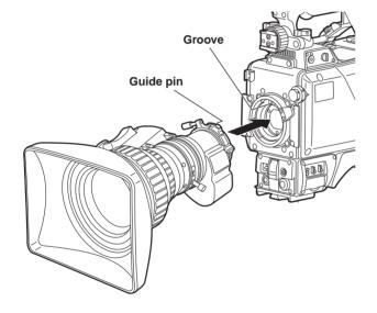
**3** Lower the lens clamp lever to clamp the lens in place.
