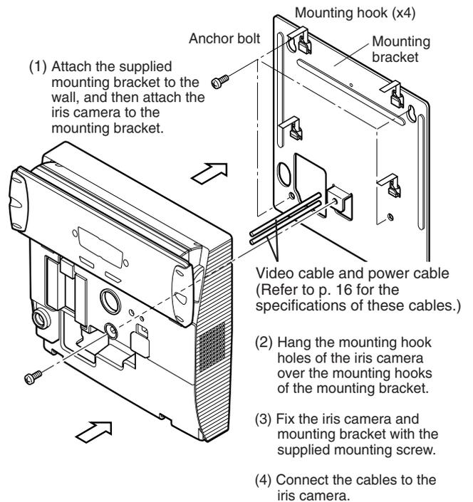
**Note:** If you lay cables along a wall surface, replace the cable hole cover on the bottom of the iris camera. (Refer to p.12.)
