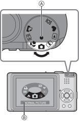
The above screen (B) appears on the LCD monitor if the mode dial is rotated. (P20) The mode currently selected appears on the LCD monitor when the camera is turned on.
