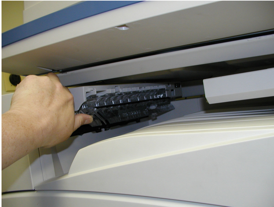
Figure 18 – Another view of the finisher’s bridge misfeed-access area.
