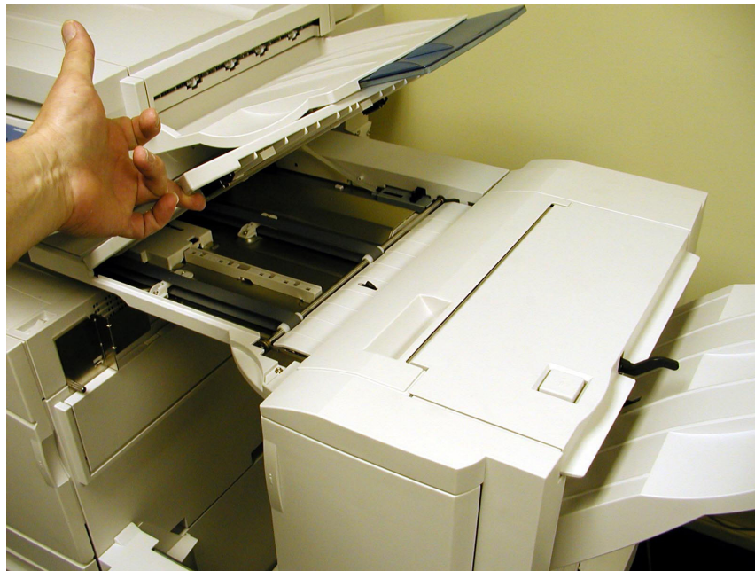
Figure 17 – The finisher's bridge misfeed-access area.
