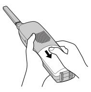
Remove the old battery. Insert the new battery into the handset as shown, matching the correct polarity (1). Press the battery down until it places into the compartment (2).
