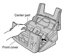
3 Clean the document feeder rollers and rubber flap with a cloth moistened with isopropyl rubbing alcohol, and let all parts dry thoroughly.
