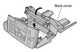
**5** Clean the thermal head with a cloth moistened with isopropyl rubbing alcohol, and let it dry thoroughly.
