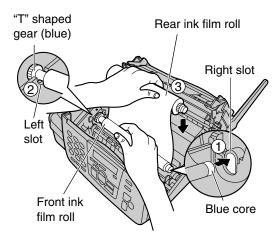
5 Turn the "T" shaped gear (blue) in the direction of the arrow.
