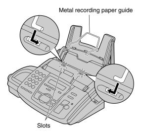
The recording paper will be ejected from the top of the unit after printing. The metal recording paper guide prevents the printed paper from curling.
