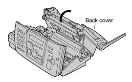
Insert the blue core of the front ink film roll into the right slot of the unit (1). Insert the "T" shaped gear (blue) into the left slot of the unit (2).
