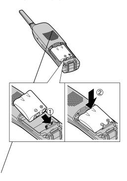
Close the cover. Make sure you charge the new battery for about 15 hours in order to display the battery strength prompt correctly (page 21).
