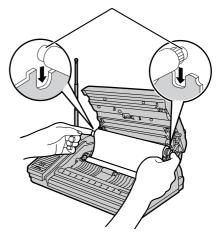
If the ink film is slack, tighten it by winding the "T" shaped gear.
