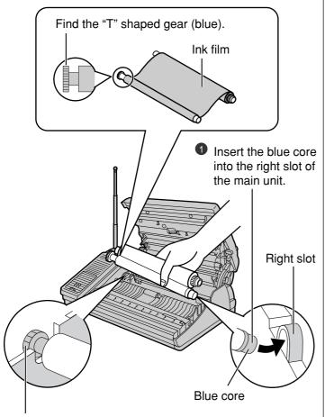
Insert the "T" shaped gear (blue) into the left slot of the main unit.
