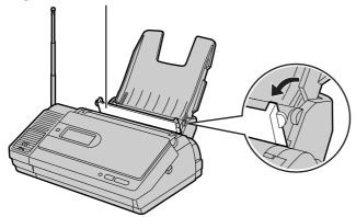
2 Fan the stack of recording paper (A4 size).
