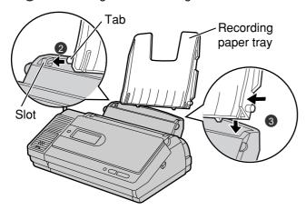
2 Insert the recording paper into the recording paper tray.
