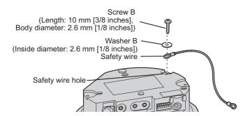
**8.** Align the 2 round protrusions on the camera and the holes on the ceiling plate (included with the camera), tighten the screw to secure the ceiling plate, then pass the safety wire through the ceiling plate as shown. Make sure you do not scratch the lens cover when performing this procedure.
