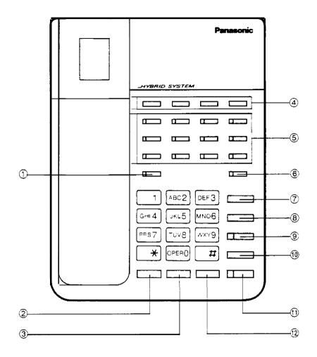
INTERCOM Button and Indicator: Used for making or receiving an intercom call.
