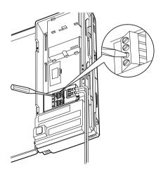
**3.** Insert the wires coming from the door openers into holes and tighten the screws.
