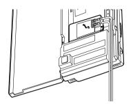
2. Loosen the screws on the terminal strip.
