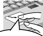
While holding down the button, moving your finger on the work surface
