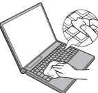
3 Slowly lift up the computer, keeping it level, and wipe any water coming out of the holes on the bottom using a soft, dry cloth
