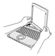
Rotate the display 180 degrees in the direction of the arrow while holding both sides.
