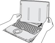
② Hold the bottom left and bottom right of the display, and rotate the display in the direction of the arrow.
