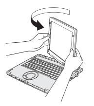
3 Rotate the display 180 degrees in the direction of the arrow while holding both sides.
