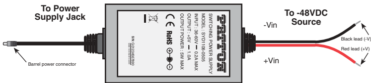
Figure 11. Connecting DC Power to the 2701 DC Power Supply.
