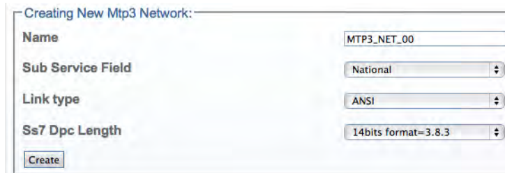
Figure 193. Creating a New MTP3 Network
