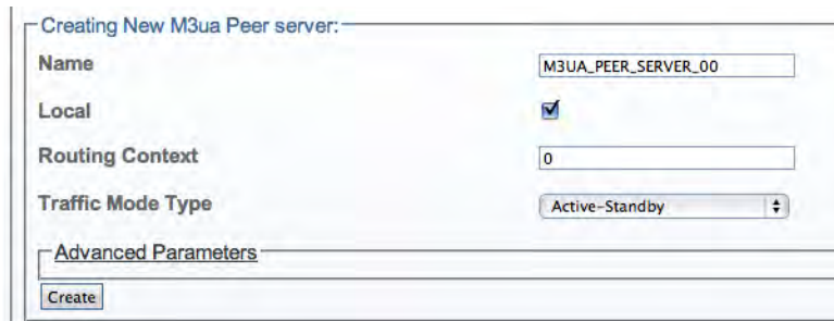
Figure 289. Creating the New M3UA Peer Server
