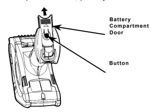
the printer, turn the printer upright, and catch the battery in your hand as it slides out.
