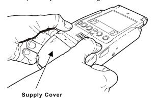
Drop the supply into the well. Make sure the supply unwinds from the top as shown.
