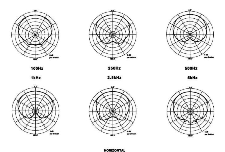
**NOTE:** Vertical polars in half-space are virtually identical to horizontal polars shown.
