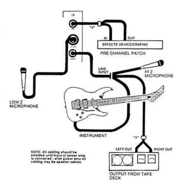
Note: Low and High impedance inputs can not be used at the same time.
