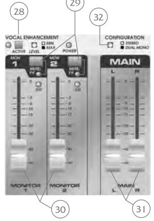
31. **MAIN LEFT AND RIGHT FADERS:** These are the master left and right faders. If the main outputs are set to dual mono, both have the same signal (sum of left and right) and can be used as zone outputs for house and annex levels etc. These controls are best operated at the 0 (full up) position. It is most important that
