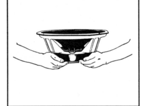
Clean the voice coil "gap" to remove any foreign matter. Fold a strip of masking tape into a small triangle with the adhesive side out for this procedure.
