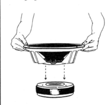
When the three screws are removed, carefully lift the magnet structure vertically from the basket assembly and flip structure over with the gap up.
