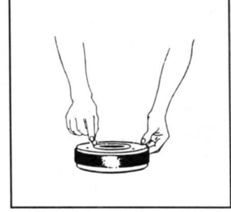
With the speaker face down, replace the three screws and tighten.
