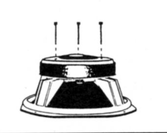
Place the magnet structure on a flat surface with the "gap" facing upward and carefuly lower the new basket assembly onto the magnet structure. Use extreme care in order to avoid damaging the voice coil.
