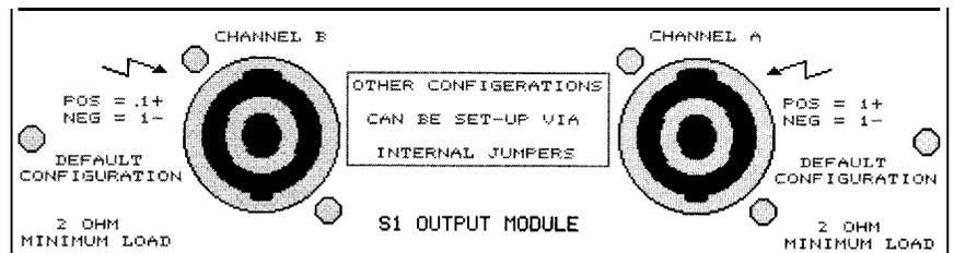
**THE S1 OUTPUT MODULE REAR VIEW LOW CURRENT STEREO MODE (18) (Option 1)**
