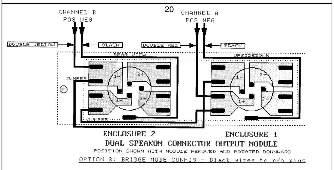
**THE S1 OUTPUT MODULE REAR VIEW - BRIDGE MODE (20) (Option 3)**
