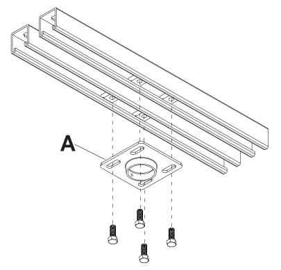
Once ceiling plate (A) is in desired position, tighten screws. When attaching the ceiling plate (A) to flush mount tube or extension column, tighten at least four complete turns ending with one of the small threaded holes aligned with slot in the end of flush mount tube or extension column. Insert and tighten one #10-32 screw (B) to lock tube position (shown below on right side).
