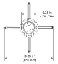
\*Mounting holes on projector must be within a 16.6" diameter in order to use this product.
