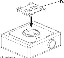
NOTE: \*Notch on interface bracket indicates front of projector.
