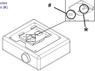
Fasten interface bracket (**K**) to adapter plate using two M5 socket-pin screws (**E**). Tighten screws (**E**) using 4mm allen wrench (**K**).
