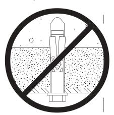
THESE CONCRETE ANCHORS ARE FOR DIRECT ATTACHMENT TO LOAD BEARING CONCRETE ONLY! NOT FOR ATTACHMENT TO CONCRETE CEILING COVERED WITH PLASTER, DRYWALL, TILE OR OTHER FINISHING MATERIAL!
