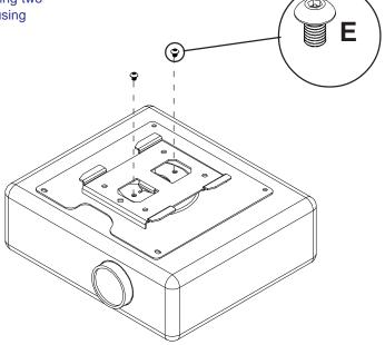
Position four tabs in interface bracket (K) behind four tabs in base unit. Slide forward to engage latch. BE SURE THAT LATCH IS ENGAGED!
