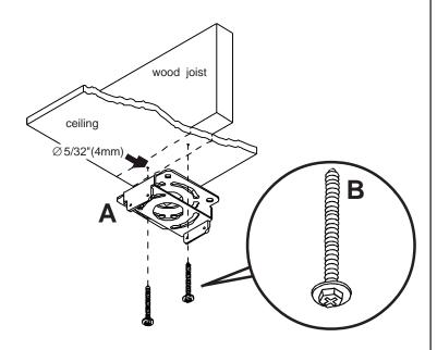
Attachment to a Wood Joist. Use a stud finder to locate ceiling joist. Drill two 5/32" (4mm) dia. holes 2.5" (65mm) deep into joist center. Attach projector mount ceiling plate (A) using #14 x 2.5" (6mm x 65mm) wood screws (B).
