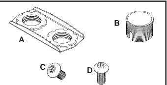
Attach adapter bracket (A) to bottom extension column (sold separately). Thread flush mount tube (B) into bracket (A) as shown until it is threaded all the way down.
