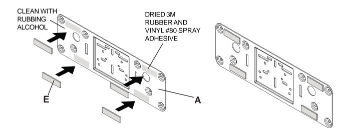
Clean desk surface with rubbing alcohol. Use 3M rubber and vinyl #80 spray adhesive (not supplied) on the <u>mounting</u> <u>surface area only</u>. NOTE: Spray adhesive <u>will not</u> remove easily. Wait at least 4 minutes to dry before removing tape backing from lock-down plate (A) and placing firmly on surface. NOTE: There is a recommended <u>72 hour cure time</u> for tape on lock-down plate (A).
