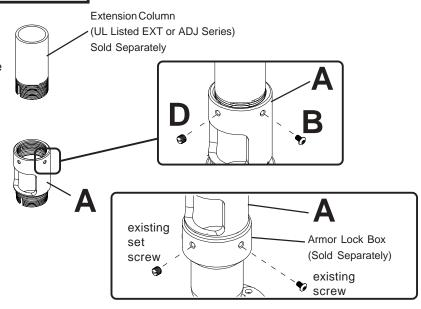
Thread cords through top of extension column and pull cords through hole in cord management adapter (A) as shown below. Note: Make sure cords are long enough to reach back of projector and not binding.
