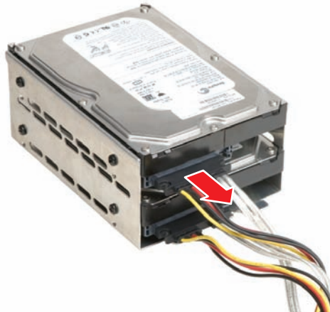
Figure 6. Removing the Power and Data Cables
