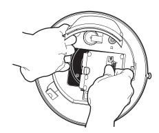
Open the hinged door to the back box. Push the tab lock towards the wall of the unit and lift the door open. Pull power, alarm/auxiliary, and network cable into the back box.
