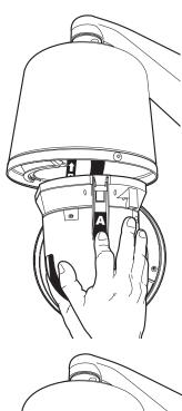
Install the dome drive. Line up the blue (A) and red (B) tabs with the blue (A) and red (B) labels. Push in the tabs. Insert one side and then the other side. Continue pushing on the ends of the tabs until both sides click into place.
