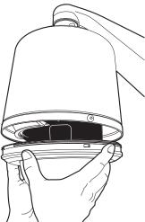
Install the lower dome. Tighten the Phillips pan head screws to secure the lower dome to the back box.
