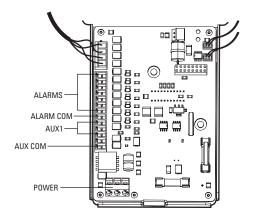
Connect a 10/100/1000BaseT network Cat5e (or better) cable to the RJ-45 network connector located inside the back box. Check the LED indicators located inside the back box to check unit status, network status, and network activity.
