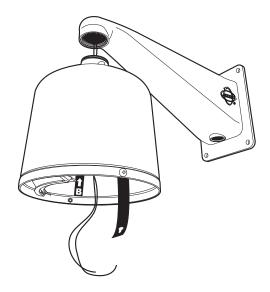
Screw the back box onto the mount. For outdoor installations, apply thread compound (provided) to the threads on the back box.
