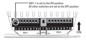
No DIP switch settings are required for the system. Before installing the dome drive verify that switch SW1-1 (SW1, switch 1) is set to the ON position and all other switches are set to the OFF position.
